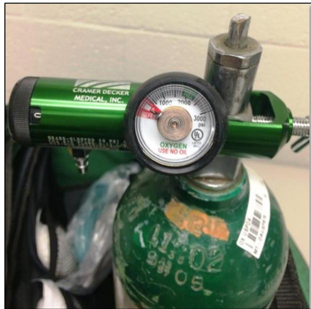
*Figure 1: Gauge showing the empty status of the EMRB oxygen tank*
