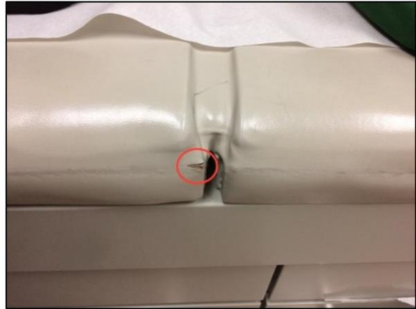
*Figure 2: Torn vinyl cover on examination table*
