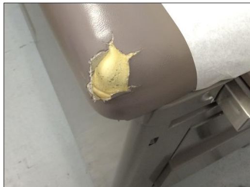
Figure 2: Torn vinyl on exam table
